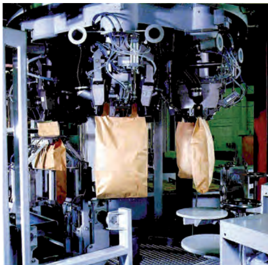
Figure 12: Modern AGFI with a high-speed packaging line and a rotating carousel (the photograph is the property of Chronos Richardson).
