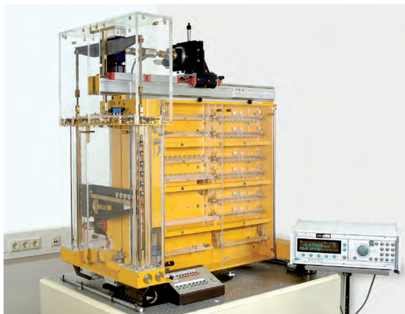
Figure 1: 1-N · m torque standard machine with a measuring range from 1 mN · m to 1 N · m
