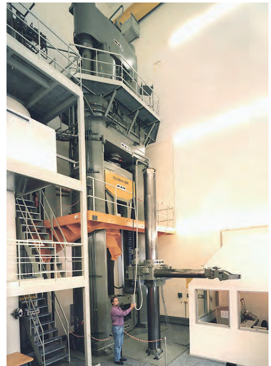
Figure 7: 16.5 MN force standard machine with hydraulic transmission
