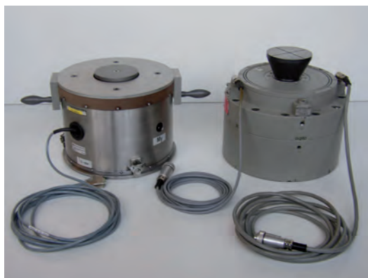
Figure 2: The 1 MN force transducers used for the 1 MN key comparison.
