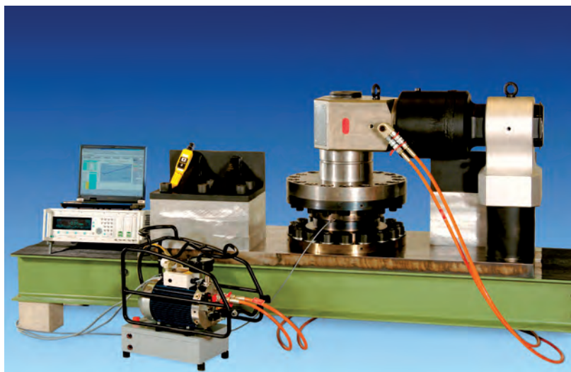
Figure 5: Hydraulic servo screw- driver up to 70 kN·m in a calibration facility
