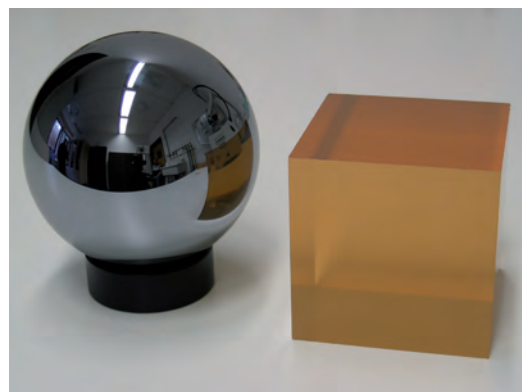
Figure 1: Examples of primary density standards: 1 kg silicon sphere and Zerodur cube
