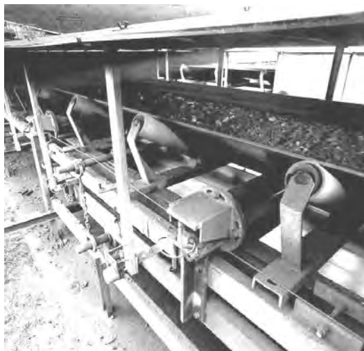
Figure 10: View of a belt weigher (the photograph is the property of Schenck Process).
