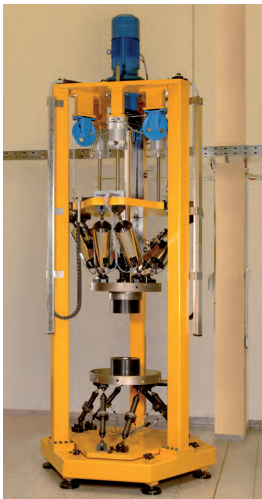
Figure 2: Multi-component refer- ence measuring machine with a force vector mag- nitude of maximum 10 kN and a moment vector magnitude of maximum 1 kN·m.
