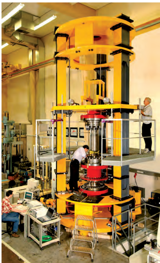
Figure 4: 1.1-MN · m torque standard machine with measuring ranges from 4 kN · m to 220 kN · m, as well as from 20 kN · m to 1.1 MN · m
