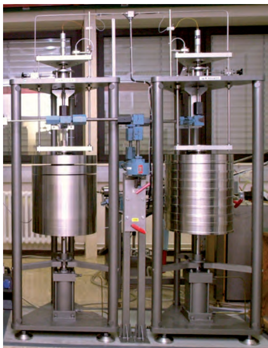
Figure 4: Standard pressure balance for the realization of the pressure scale in liquids in the range from 0.5 MPa to 1 GPa.
